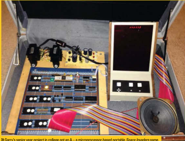
» Garry's senior year project in college got an A – a microprocessor-based portable Space Invaders game.
